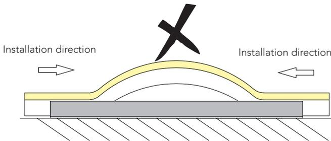
Incorrect installation like below picture could lead to light failure.
