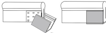
3. Insert the rubber gasket along the slit into the pin of the front connector
