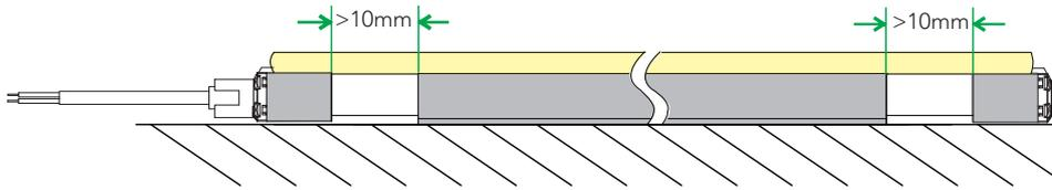
Press the flex light into mounted aluminum channel in one direction.
