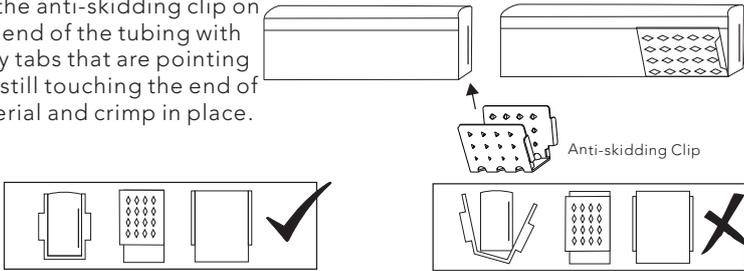
2. Line up the aluminum mounting piece so the screw holes face the plug and slide on over the anti-skidding clip.
