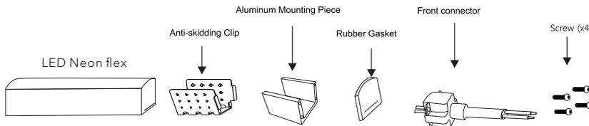
1. Place the anti-skidding clip on the very end of the tubing with the 2 tiny tabs that are pointing inwards still touching the end of the material and crimp in place.
