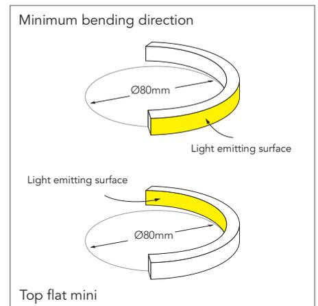
LED Neon flex is a highly durable product but must be installed in accordance to the pictures shown below, which indicate the minimum bending parameters as well as the correctly bending direction for each specific variant of model
