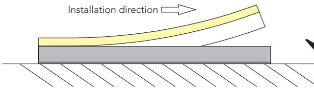
Do not bend against light terminals; otherwise it will lead to failure of connector waterproof.
