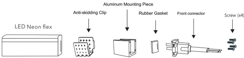
1. Place the anti-skidding clip on the very end of the tubing with the 2 tiny tabs that are pointing inwards still touching the end of the material and crimp in place.
