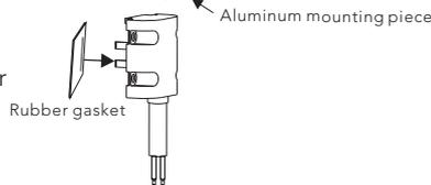
4. Put 100% clear silicone on the surface of rubber gasket
