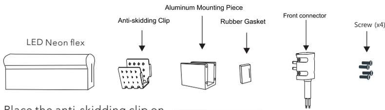
1. Place the anti-skidding clip on the very end of the tubing with the 2 tiny tabs that are pointing inwards still touching the end of the material and crimp in place.
