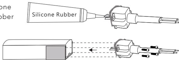
5. Carefully insert the pins of the front connector into the gap you created behind the PCB.
