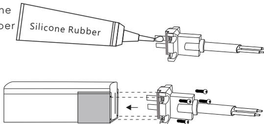
5. Carefully insert the pins of the front connector into the gap you created behind the PCB.
