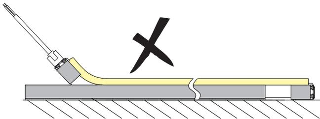
Ensure the feeding cable not bear force, keep the head 10mm in natural loose.
